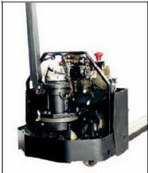
WP20M Internal Structure: DC vertical driving motor standard, AC vertical driving motor optional.
